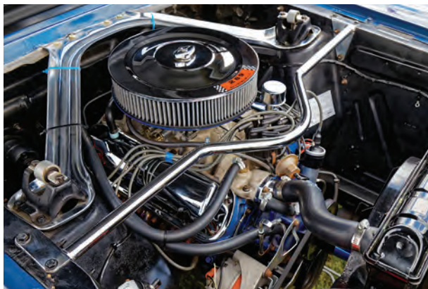
The '65 Mustang's 4,700cc engine. Photo: Acabashi
